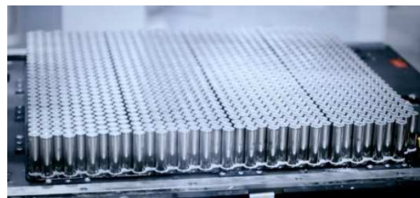
Figure 4. Tesla Model S - Lithium-Ion Battery
