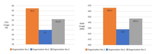
Figure 4. Consumption of processor and operation memory (RAM) during rendering process
